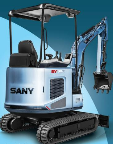
As well as zero emissions and considerably lower noise levels, the compact electric SY19E is equipped with a lithium iron phosphate (cobalt free) battery which allows for faster, safer and more efficient charging as well as a significantly longer battery life to reduce total cost of ownership.
