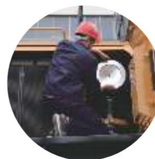
Replace air filter element
