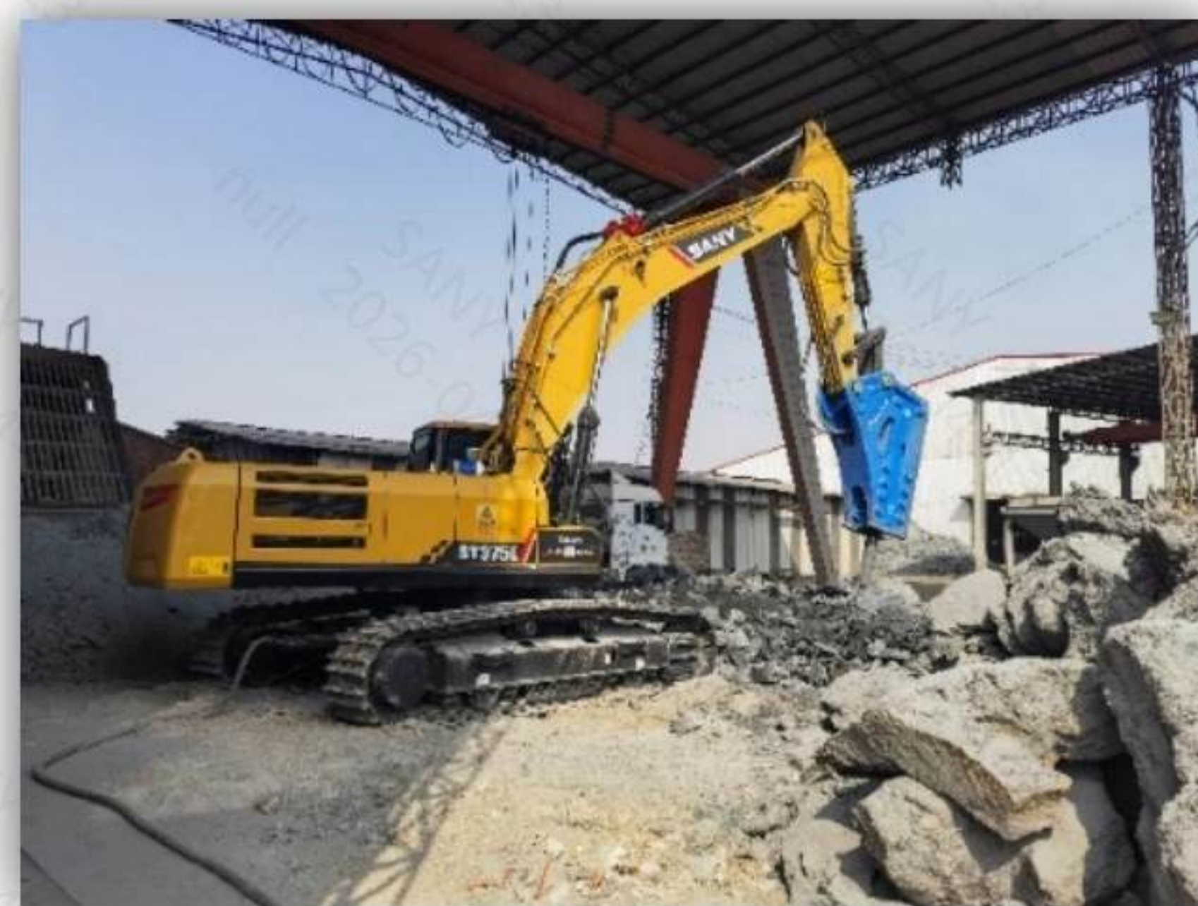
SY375E work with 175mm breaker
